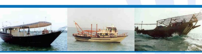
Piviera has deep regard for history. It is our rich legacy of the past that steers us towards success in the future. Riviera pioneered in fibre glass dhow building (GRP) in the Middle East. According to individual needs Riviera can make Dhows ranging from 45 feet to 90 feet. The Dhows are built for various applications and with different specifications to satisfy client requirements.
